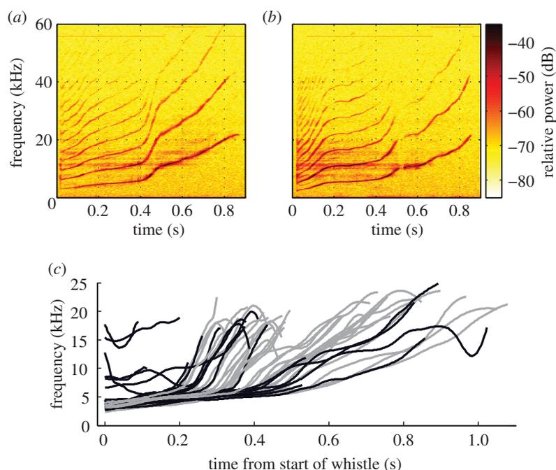
Figure 1. (a) Tonal call produced breathing air. (b) Tonal call produced breathing heliox. (c) Fundamental frequency contours of tonal calls produced while breathing air (grey,  $n = 34$ ) and heliox (black,  $n = 19$ ).
